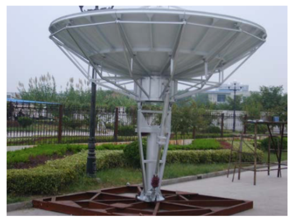
(Non penetrating foundation)
